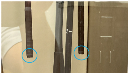
Figure 1: Damaged glue joints on the bending section
