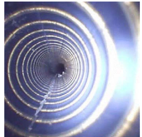
Figure 2: Scratched endoscope channel
