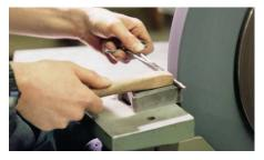
**Step 8: Bending.** The bending step involves the use of specialized tools to bend an instrument (i.e., the jaw of an atraumatic clamp) to ensure the correct shape is consistently achieved.
